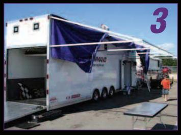
Install awning cover and connect to zipper flap. Cover installation can be performed using ladders from the ground or from the roof of the trailer.
